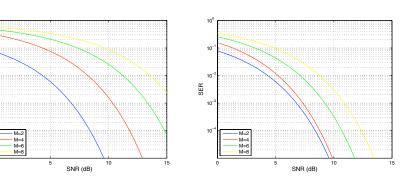
The energy required for a target  $P_e$  increases with the cardinality M
