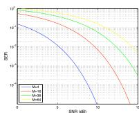
The energy required for a target  $P_e$  increases with the cardinality M
