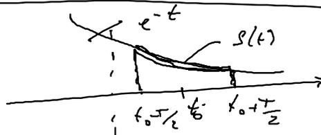
$$S(f) = \int_{t_0 - T/2}^{t_0 + T/2} e^{-t} e^{-j2\pi f t} dt$$
