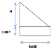
$$\int_0^b |y(x)|^2 dx = \frac{H^2 \cdot \text{BASE}}{3} + (H + \text{SHIFT}) \cdot \text{BASE} \cdot \text{SHIFT}$$
