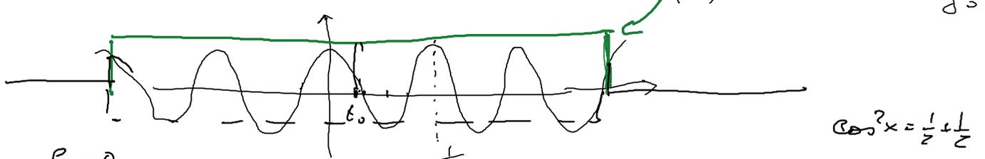
$$E_s = \int_{t_0 - T/2}^{t_0 + T/2} \cos^2 2\pi f_0 t \, dt = \int_{t_0 - T/2}^{t_0 + T/2} \frac{1}{2} dt + \frac{1}{2} \int_{t_0 - T/2}^{t_0 + T/2} \cos 4\pi f_0 t \, dt$$
