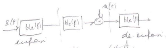
$$\begin{cases} |H_e(s)|^2 = \frac{K \alpha}{|H_d(s)|} \left( \frac{P_u(s)}{P_s(s)} \right)^{1/2} & \text{const.} \\ |H_d(s)|^2 = \frac{K}{\alpha} \frac{1}{|H_e(s)|} \left( \frac{P_s(s)}{P_u(s)} \right)^{1/2} & \text{const.} \end{cases} \quad f \in [b, B]$$
